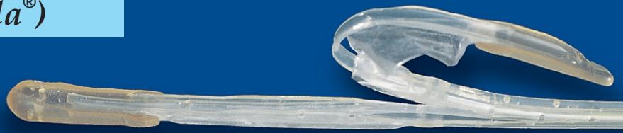
Force exerted on air-filled balloon at the tip is mechanically transmitted through an air column to remote transducer. The reused electronic pressure transducer located in the end of the interface cable converts mechanical pressure signal to electrical signal for fetal monitor.
